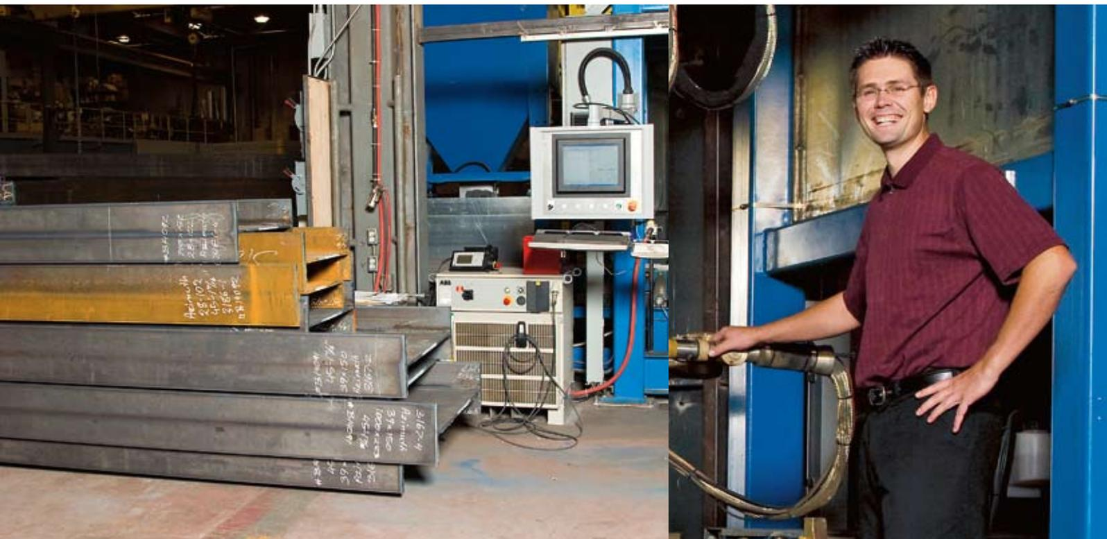
and slots and cutting copes in mere seconds. By contrast, hand cutting can take 10 minutes or more when you factor in the measuring. Many shops still use pencil and paper to interpret from blueprints where holes have to be cut. That process is slow and prone to misinterpretation of designers' specs. And then there's the shortage of workers, a situation that is getting worse, Diab says. Kwiatkowski's robot can even compensate for those minor variations in the dimensions of the steel beams.
